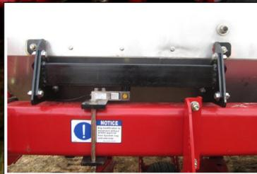
Close-up of **Load cell** mounted with brackets to main frame to support the hopper and weigh applied product.
