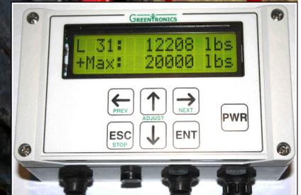
**Controller** with sealed keypad and bright display to show application data and to navigate the simple menu system.
